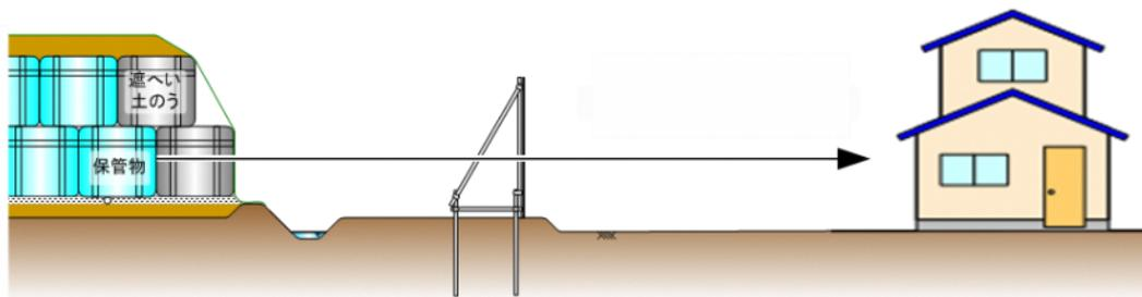
FIG 4.4. Typical layout for a TSS. Radiation doses are calculated with respect to the distance from stored materials (Image: Fukushima Prefecture).
