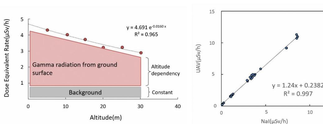
Fig. 5.3. On the left: illustration of exponential dependence of the dose equivalent rates measured by the UAV-based system and represented as a function of altitude. On the right: illustration of linear dependence of UAV data obtained with Geiger-Müller counter with respect to reference NaI data (both measurements were performed at 1 m altitude and for different dose equivalent rates). Image: Fukushima Prefecture.
